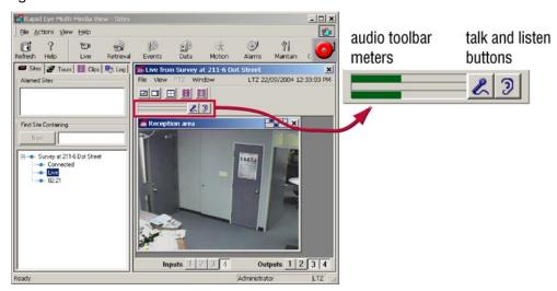
Fig. 3. Audio toolbar for a Multi-Media LT unit, when using View.
